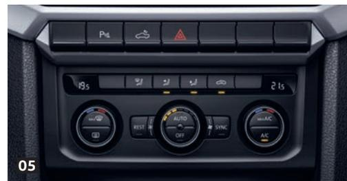
**05 Climatronic air conditioning.** This system offers 2-zone temperature control for the driver and front passenger. Depending on the intensity of the sun's rays and the outside temperature, the air conditioning adds more or less cool air accordingly.
