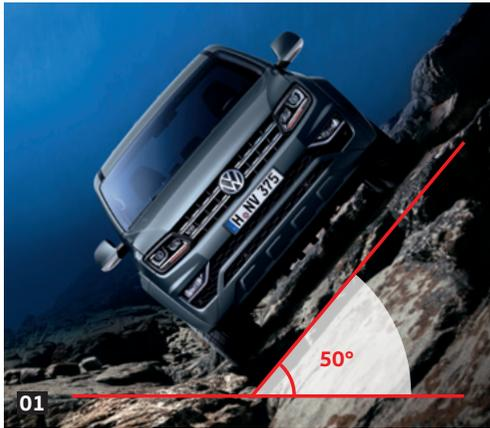
**01 Side slope angle.** The broad track of the Amarok provides enormous stability even when driving along slopes with up to a 50° incline.<sup>1</sup>
