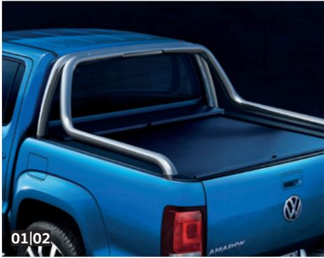
**01 Roll cover.** The lockable load compartment cover protects the cargo from prying eyes. Accessory
