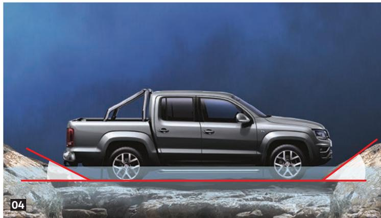
**04 Approach/departure angle and wading depth.** The maximum slope angle for the new Amarok is 28.0° at the front and 23.6° at the rear. It can handle pool with a wading depth of 500 mm.
