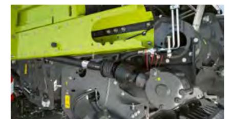
Metering roller drive.
