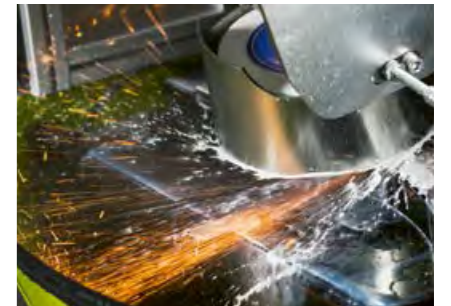
Because the grinding angle is always correct, the original radius and contour of the knives are maintained.
