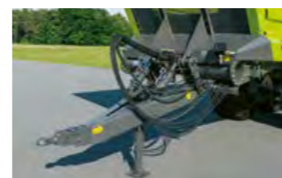
The articulating drawbar is operated via two large double-acting rams.
