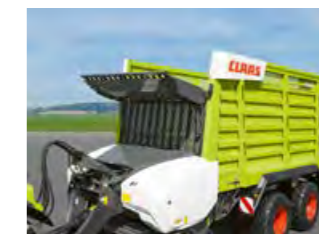
Filling flap folds hydraulically towards the front.
