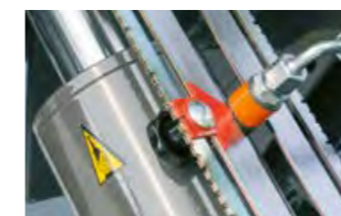
Marker arrow for the horizontal position of the articulating drawbar.
