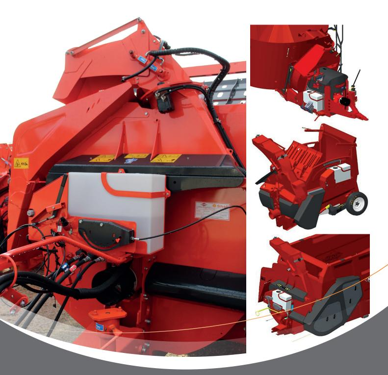
The CLEANSTRAW system is available on all Kuhn turbine machines (straw blowers, silage cutters + straw blowers and mixers with straw-blowing function). It uses added water to minimise suspended dust in buildings during straw blowing.
