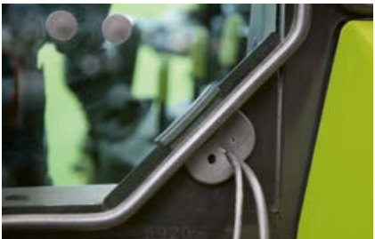
The cable feedthrough on the rear window provides different hole sizes for most cables.
