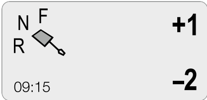
REVERSHIFT progressivity setting in the CIS
