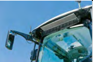
Easy access to the cab air filter on the cab roof
