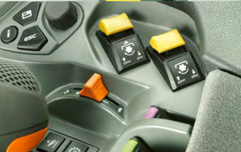
External controls for front and rear PTO
