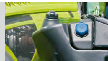
700 l fuel tank with integral 60 l urea tank
