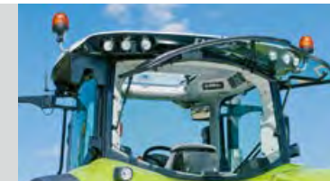
The convex rear window has a wide opening angle.
