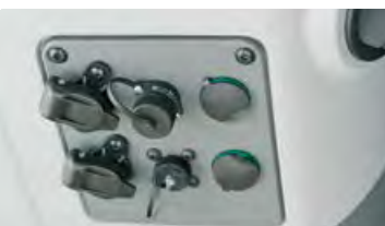
Connections to the power supply (25 A and cigarette lighter) and ISOBUS for additional terminals are located below the right-hand console.
