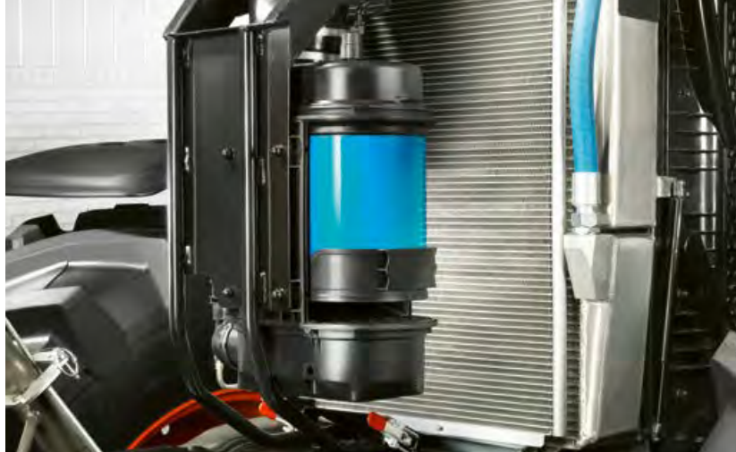
Easy access to the cab air filter on the cab roof
