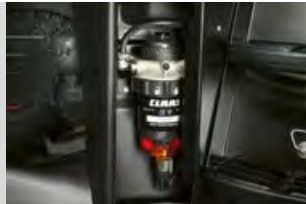
The fuel pre-filter is conveniently located by the steps to the cab.
