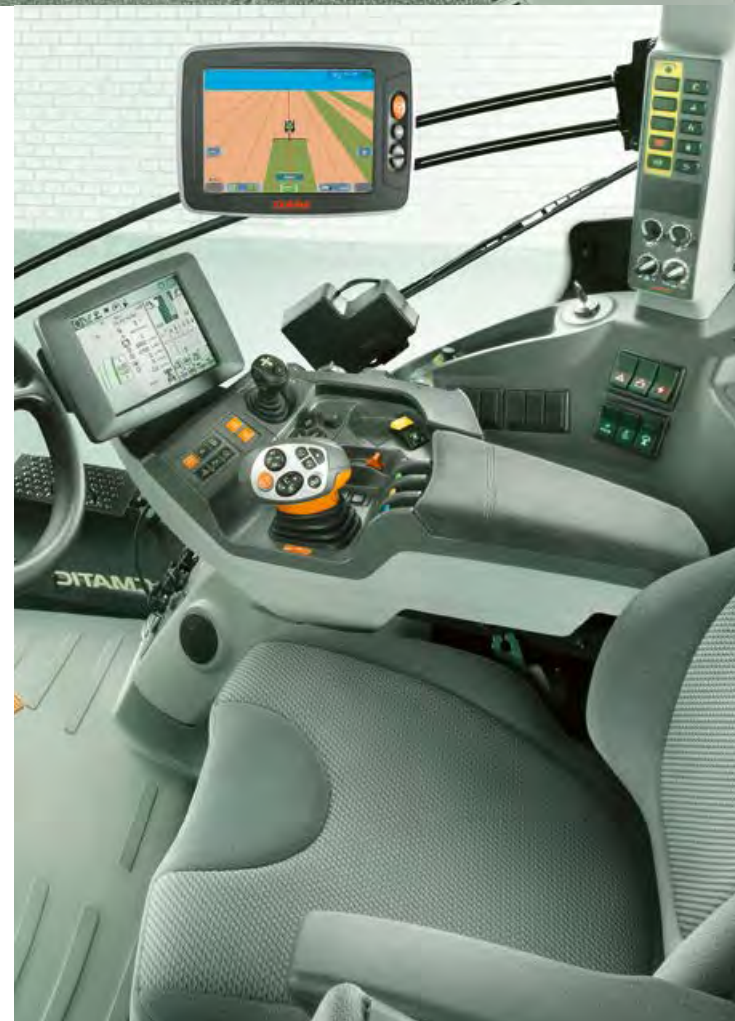
Control panel (11) in the armrest: four-wheel drive, differential lock, automatic PTO engagement/disengagement and front axle suspension
