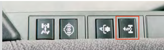
Switch to activate front axle suspension
