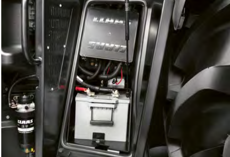
The fuel pre-filter is conveniently located by the steps to the cab.
