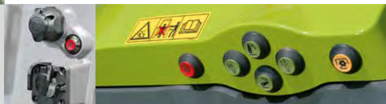
External controls for front and rear PTO
