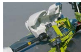
Hydraulic clutch for sequential actuation of auger and mowing bar
