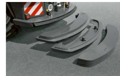
The flexible rear ballast also provides the JAGUAR with a wide collision protection element
