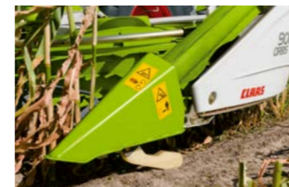
AUTO CONTOUR, ground pressure control with lateral levelling
