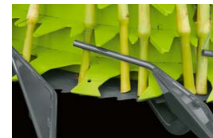
Gentle crop transport and self-sharpening effect
