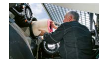
Air filter change without tools
