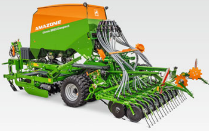
Cirrus 3003 Compact with TwinTeC + double disc couler
