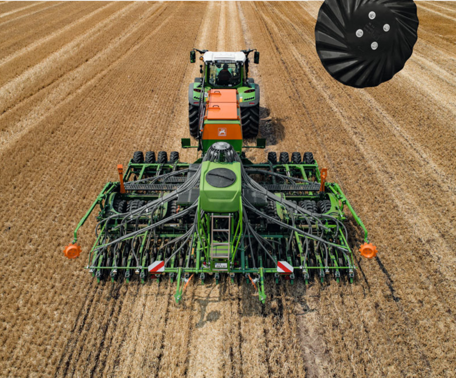
Minimal, water-conserving soil tillage in strips with the Minimum TillDisc
