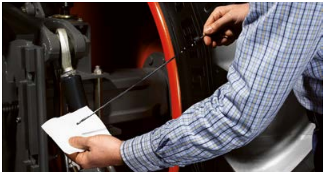
It's easy to check the transmission oil level at the rear.
