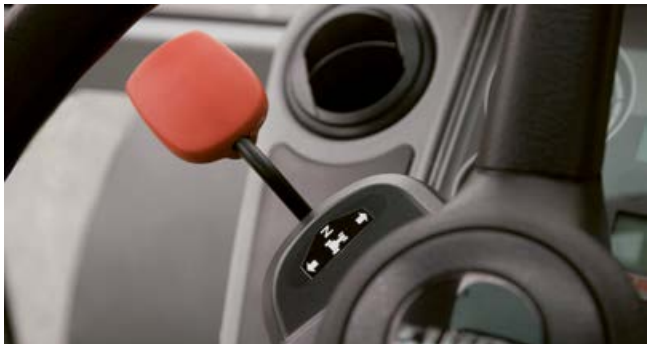
Operate the REVERSHIFT clutchless reverser with your fingertips.
