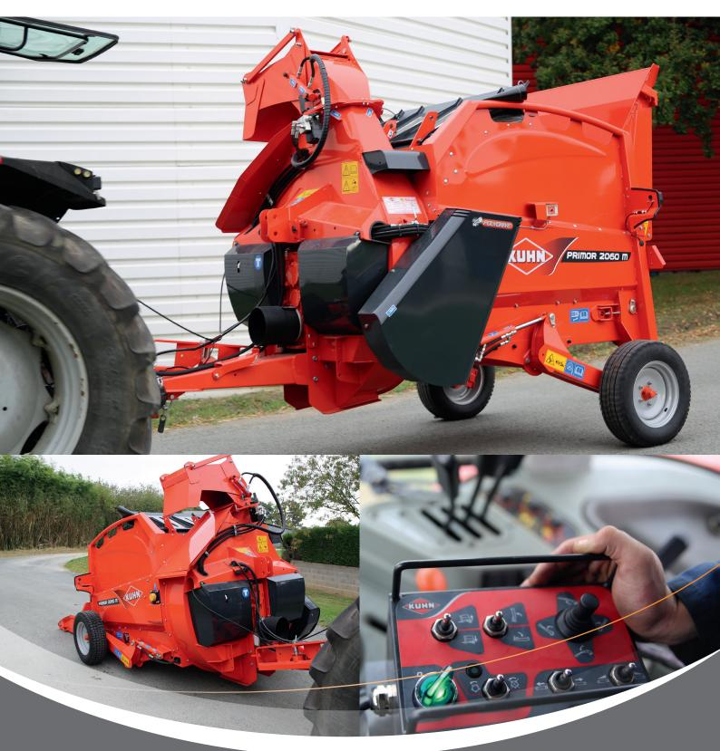
The PRIMOR 2060 M semi-mounted version is an additional model to the straw blower and all-fodder feeder range with a **new model adapted for low-power tractors requiring fodder distribution**. This machine allows to load either one rectangular bale (up to 1.30 m x 1.20 m x 2.70 m), or 1 round bale (up to 1.80 m in diameter) independently with an adjustable axle mounted on two cylinders.
