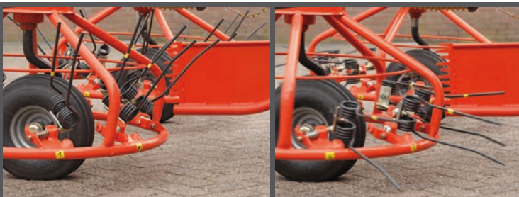
Centrifugal force controlled tines
