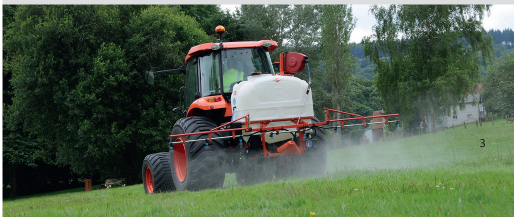
RPL 12 m/ 24 nozzles - 3 sections - safety springs, protected nozzles, link suspension (option), manual or hydraulic hoist (option)
