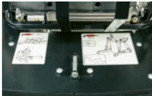
A lubrication chart under the bonnet simplifies maintenance
