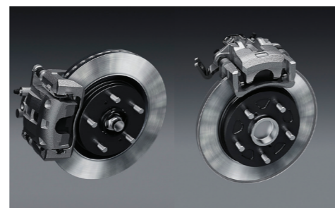
16-inch ventilated front disc brakes 15-inch solid rear disc brakes
