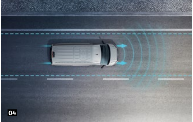
04 Lane Keep Assist*. Countersteers if a lane is left unintentionally while alerting the driver at the same time by using a warning tone and information in the multifunction display. | KS | KA |
