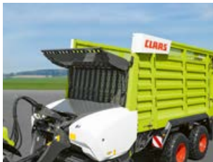
Filling flap folds hydraulically towards the front.
