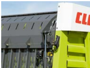
Angle sensor on the filling flap.
