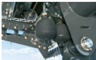
Accumulator for the optional drawbar suspension.
