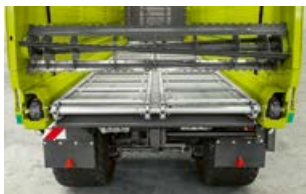
Two powerful hydrostatic motors, in combination with the two-speed drive, guarantee rapid discharge.
