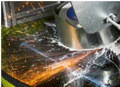
Because the grinding angle is always correct, the original radius and contour of the knives are maintained.
