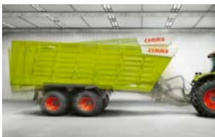
The hydraulic articulating drawbar allows the entire wagon to be raised or lowered to its maximum and minimum heights.
