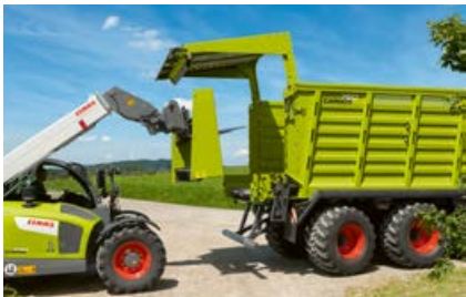
Rapid module assembly for higher loading volume and weight reduction of about 500 kg.
