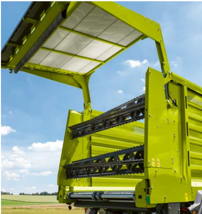
Rapid module assembly for higher loading volume and weight reduction of about 500 kg.
