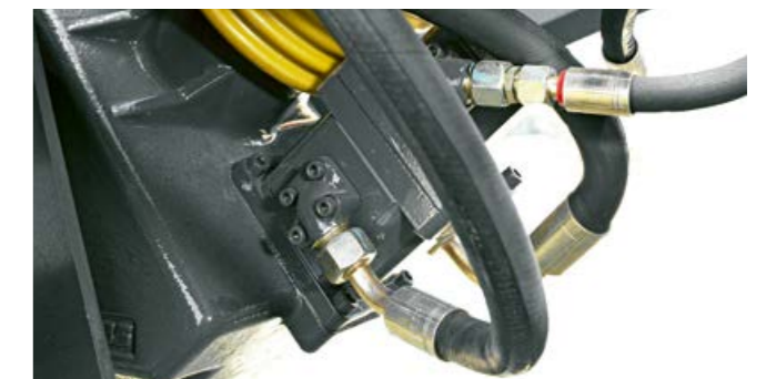
Two oil pumps supply hydraulic oil to the input transmission and the TURBO FAN knotter cleaning system
