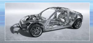
The passenger safety cell absorb and direct impact force around the cabin, rather than through it.
