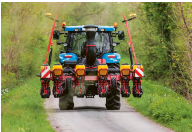
Tempo T has a transport width between 3.3 and 3.5 metres. This gives a small turning radius and convenient transport.
