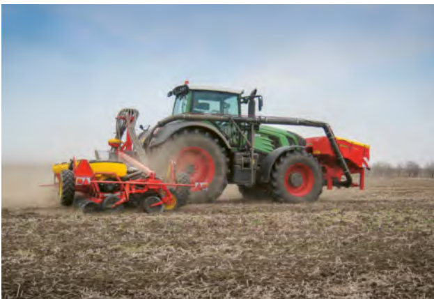
The front mounted fertiliser hopper FH 2200 enables high precision combi-drilling.
