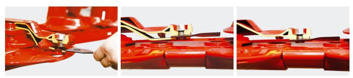
Exchanging a FAST-FIT knife quickly
