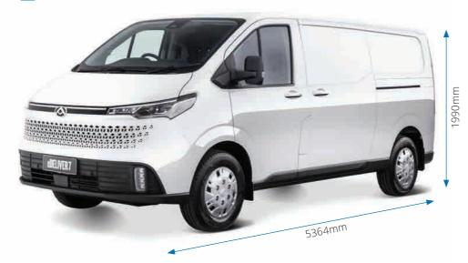
With four models on offer, you can choose the eDeliver 7 that's best for your business. Take on whatever the day throws at you with the 5.9m³ cargo volume and 1350kg payload of the short wheelbase/low roof model or step it all the way up with a massive 8.7m<sup>3</sup> cargo volume and 1175kg payload of the long wheelbase/high roof model.
