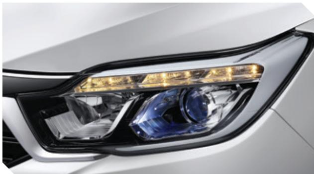
Elegant front light cluster with high-intensity-discharge headlamps for excellent night vision; LED daytime running lights, positioning lamps and directional indicators
