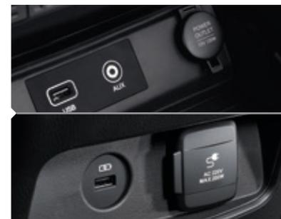
USB port and power outlet on centre console, USB port and 220V/115V inverter in 2<sup>nd</sup> row
