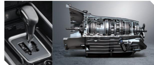
E-Tronic 7-speed automatic transmission (diesel engine)
