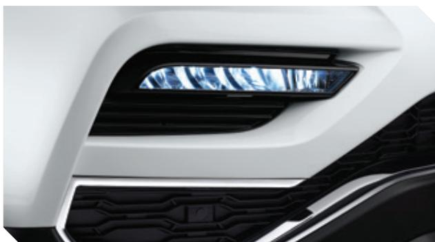
Clever LED cornering light function integrated into front fog lamps
