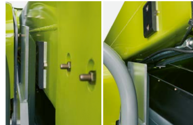
Side support for the telescopic arm is standard in the SCORPION 756 / 746.
