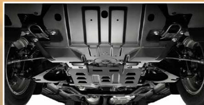
Steel underbody guards on sump and transfer case on 4x4 models
