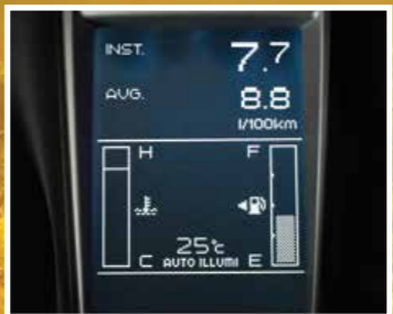
Multi Information Display of instant and average fuel consumption
