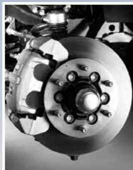
Large front brakes with ventilated disc
