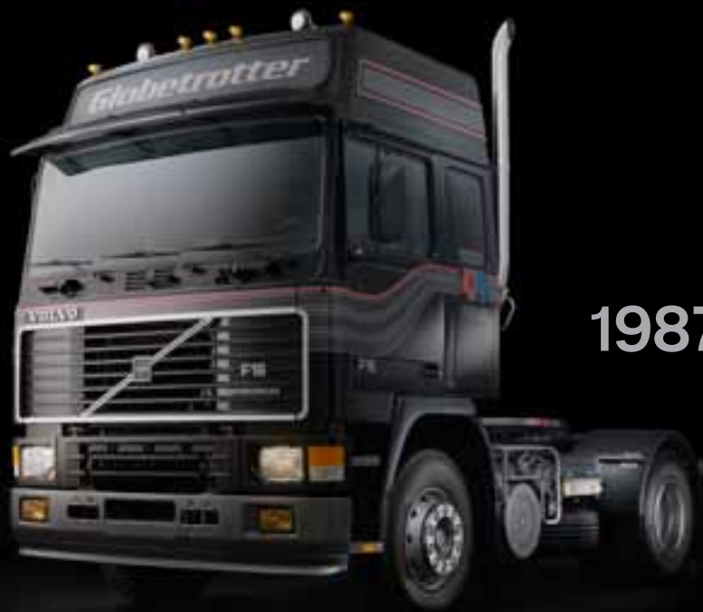
1987 – F16: Introduction of the TD162F. Unique for its superior torque, 16-litre engine volume and 6 in-line cylinders.
