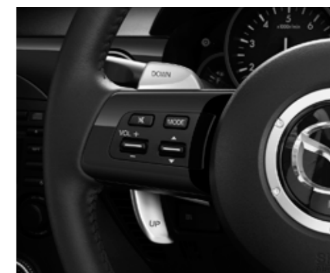
Press to play. Activematic's steering wheel paddle-shifters let you change gear with a flick of the fingertips.
