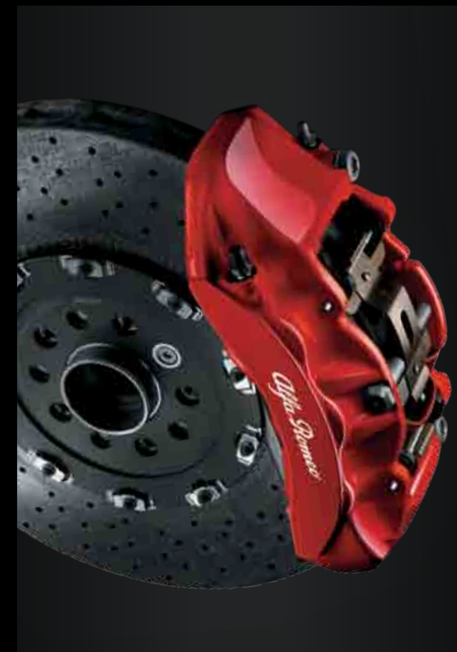
Red (Standard), Yellow (Optional)* or Black (Optional)* Calipers. Carbon Ceramic Brake Disks (Optional)* shown.
