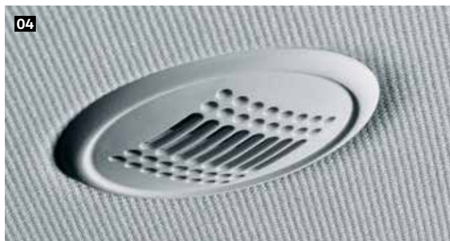
04 Electronic voice amplification. This ensures that the driver does not have to speak loudly in order to talk to the passengers in the rear compartment. The voice input is recorded through a hands-free microphone, amplified, and then transmitted over the loudspeakers in the rear. | CL | HL | EX |
