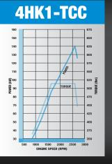
4HK1-TCC produces 140kW power and 513Nm torque on selected NPR models and is standard on NQR models.
