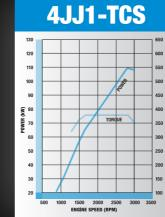
4JJ1-TCS produces 110kW power and 375Nm torque and is standard on NLR, NLS and NNR models.
